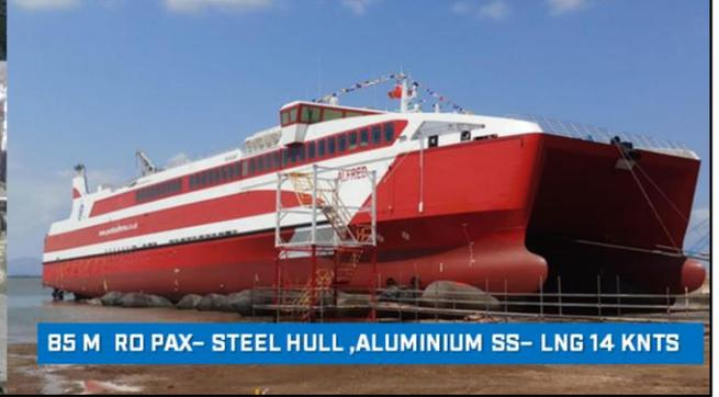
**85 M RO PAX- STEEL HULL ,ALUMINIUM SS- LNG 14 KNTS**
