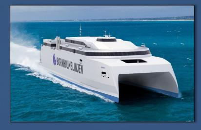
A contract for a 115 metre high speed catamaran ferry for Molslinjen of Denmark was awarded Oct 2019. At construction, it will be the largest vessel (by volume) built by Austal and has the ability to be converted to LNG fuelled propulsion.
