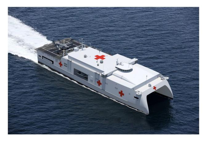
The Expeditionary Medical Ship (EMS) is a high-speed aluminium catamaran based on the proven Expeditionary Fast Transport design that offers enhanced medical support to the United States Navy. (Image: Austal USA)
