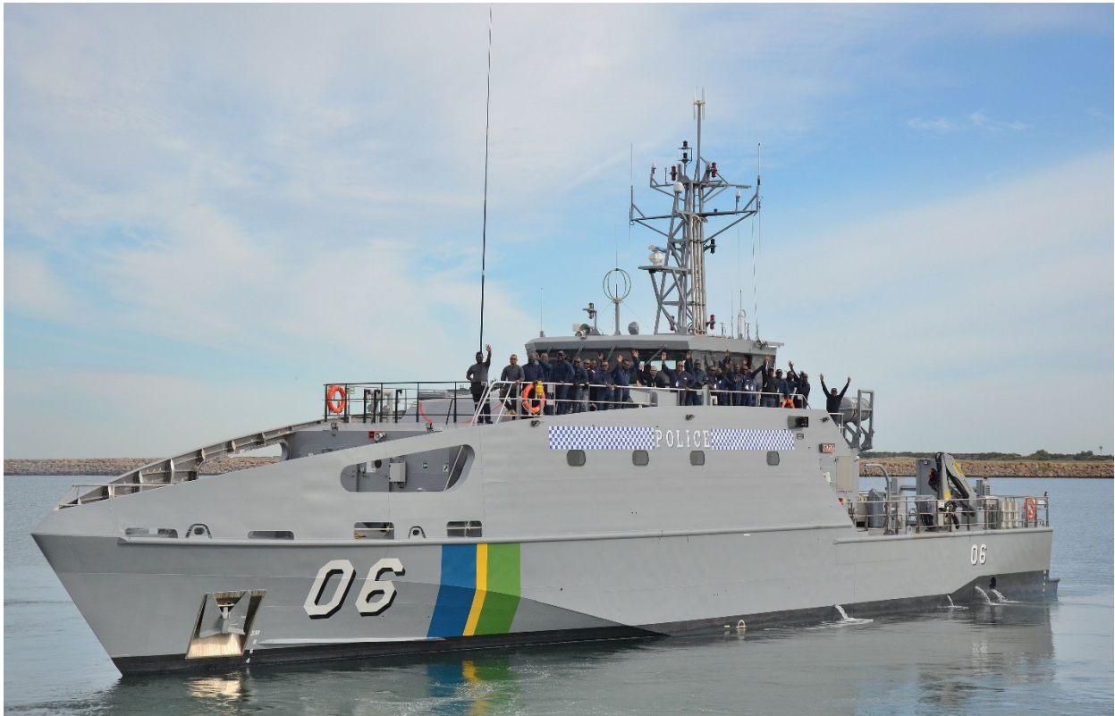
The RSIPV Taro is a 39.5 metre Guardian Class Patrol Boat, designed and constructed by Austal Australia. (Image: Austal)
