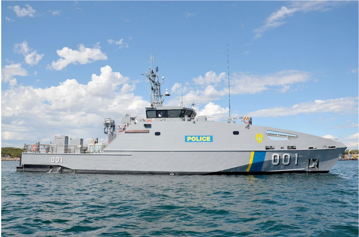
The PSS President Hi.I Remeliik II is a 39.5 metre Guardian Class Patrol Boat, designed and constructed by Austal Australia. (Image: Austal)
