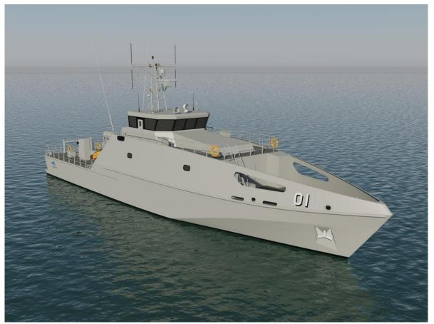
Austal's Pacific Patrol Boat Replacement Project is on schedule, with Detailed Design Review (DDR) completed on time and in accordance with the contract. Construction of the 19 steel vessels is due to commence, on schedule, in April 2017. (Image: Austal)
