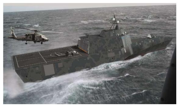
The success in operation of the Fred. Olsen, S.A. trimaran enforces our confidence in the suitability of our Littoral Combat Ship (LCS) design for the US Navy, which is based on the 127 metre trimaran hull platform.
