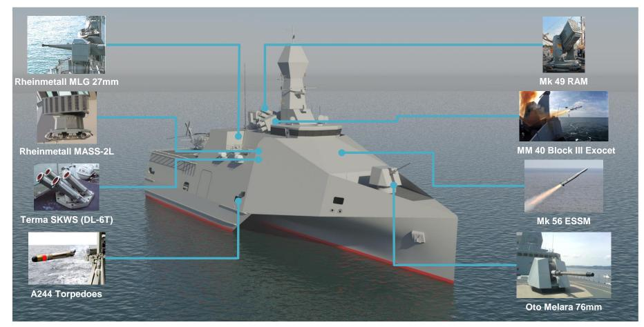
Austal's design of a smaller frigate-size multi-mission combatant that has significant capability and lethality
