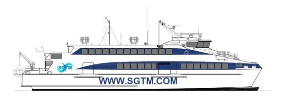
The Passenger Express 41 to be constructed by Austal's shipyard in Vietnam will accommodate 400 passengers and 20 tonnes of cargo over 2 decks. (Image: Austal)
