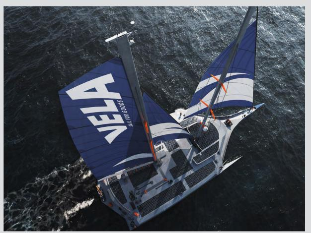
innovation and sustainability in maritime transport. In 2024, Austal Australasia was contracted by VELA, designer and operator of newgeneration sailing cargo vessels, to design and construct a 66.8-metre aluminium cargo trimaran. The trimaran will be capable of transporting high-value goods across the Atlantic Ocean using 100% wind power, drastically reducing its carbon footprint compared to conventional diesel-powered cargo ships. The vessel's shallow draft allows it
