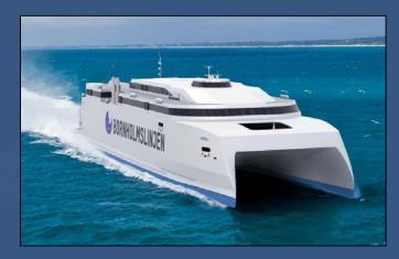
A contract for a 115 metre high speed catamaran ferry for Molslinien of Denmark was awarded Oct 2019. At construction, it will be the largest vessel (by volume) built by Austal and has the ability to be converted to LNG fuelled propulsion.
