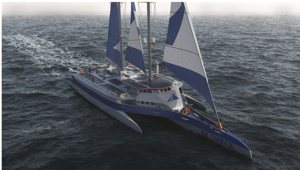
Austal is constructing a 66 metre aluminium sailing cargo trimaran for Vela Transport of France (Image: Vela Transport)
