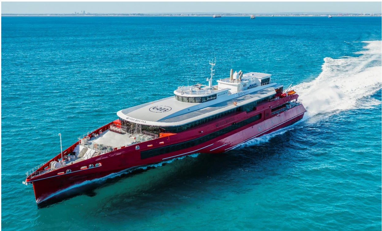
Queen Beetle is an 83 metre high speed trimaran ferry designed and constructed by Austal Australia in Henderson, Western Australia (image: Austal)
