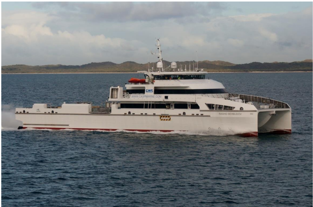
Rashid Behbudov, a 70 metre offshore crew transfer vessel constructed by Austal for Caspian Marine Services of Azerbaijan (Photo: Austal)
